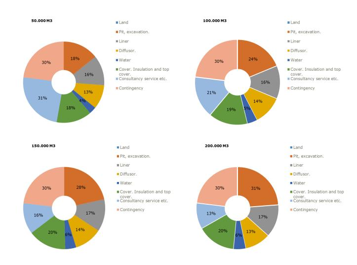
Fig. 3: Cost break down of the pit storage on a size basis
