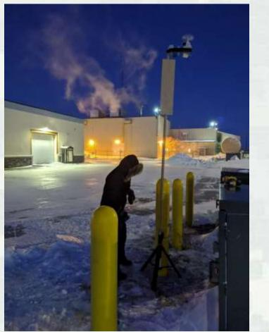
Buildings were instrumented with temperature and relative humidity sensors. Weather stations were used to obtain exterior temperatures and wind conditions.
