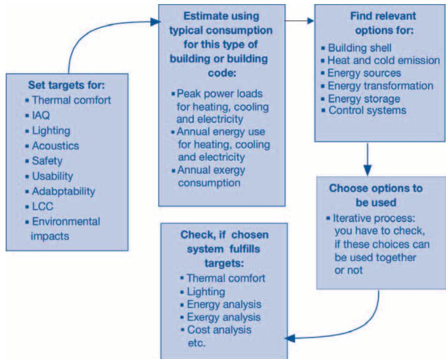
The design process is or at least should be an iterative process. There will always be a need to go back to earlier step and revise the choices made. The design process is described in Figure 23. The terms in the boxes are more explained in chapter 4.4 of the Guidebook.
