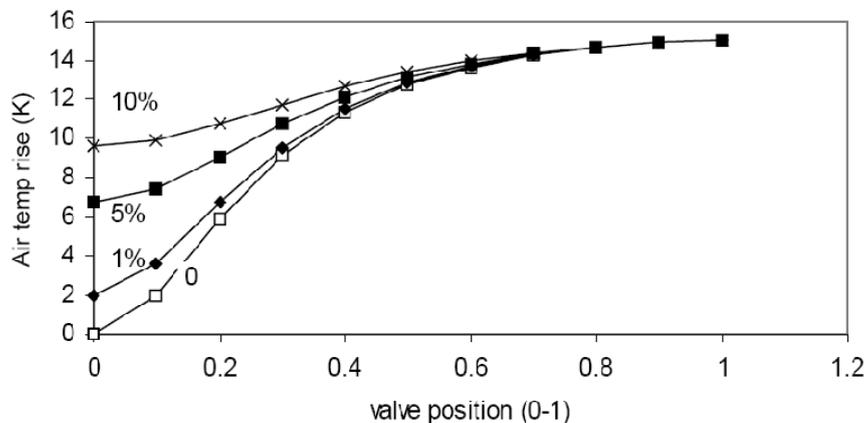
Figure 7: Heating coil air temperature rise as a function of valve position
