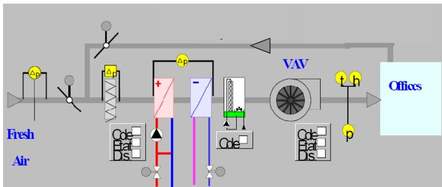
Figure 4: General view of a typical air distribution system.
