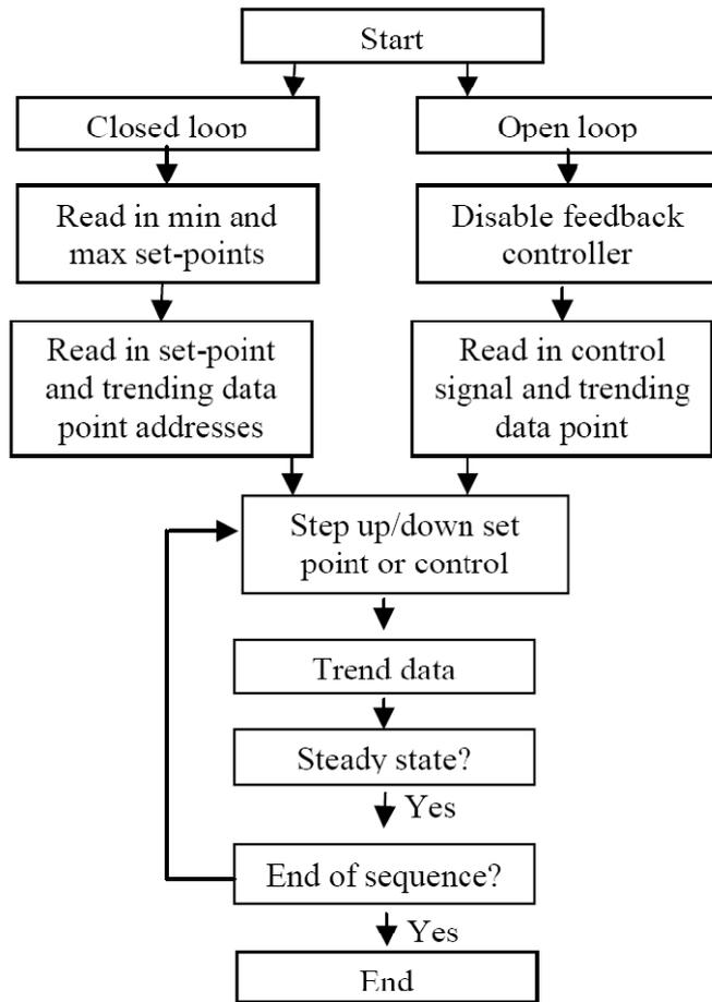
Figure 8b: Automated test signal generator.
