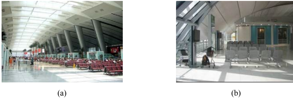
Fig. 3-25 Direct solar radiation in a large space building: (a) ceiling; and (b) sidewall.
