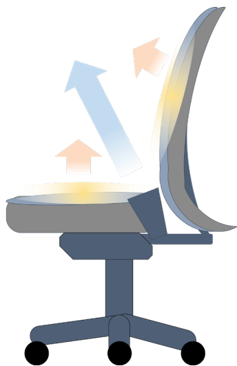
A generic example of a chair-based personalized heating, cooling, and ventilation system Source: EBC Annex 87
