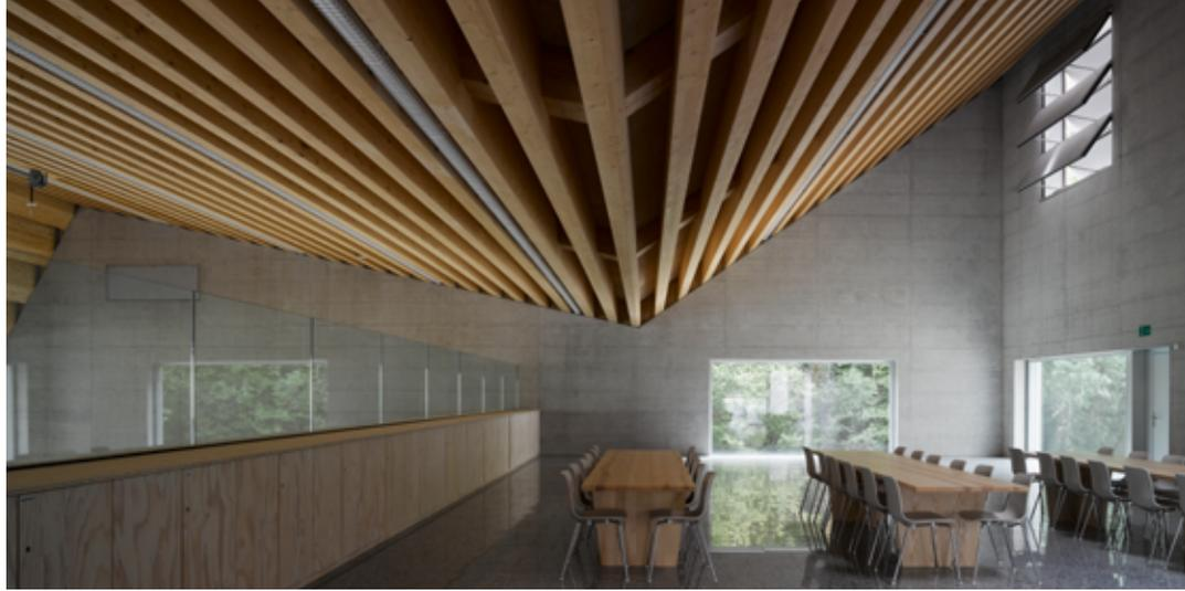
The gym and canteen at Saviese primary school in St-Germain, Switzerland, equipped with demand controlled natural ventilation and a ventilative cooling system. The monitoring results show that four groups of openings, placed at the right positions and controlled with a simple BMS system, offer excellent indoor air quality and summer comfort without the presence of a single fan or duct.
