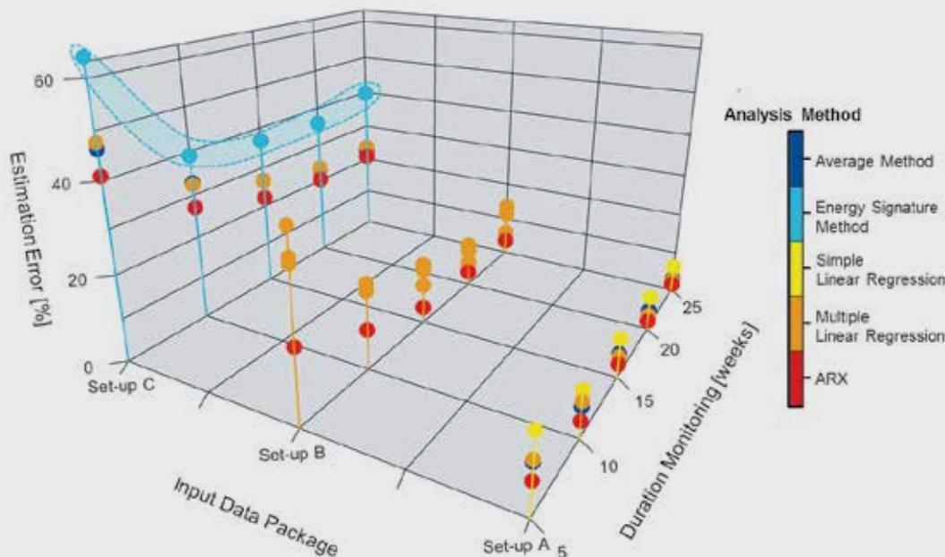
Exploration of different methods to determine the actual heat loss coefficient of a detached dwelling with slab on ground based on in-use data. The accuracy that can be achieved by each of the methods is evaluated as a function of the available data (data packages) and monitoring time. Based on this kind of graph, a motivated choice can be made regarding data package and monitoring time for a specific application with its corresponding required accuracy.
