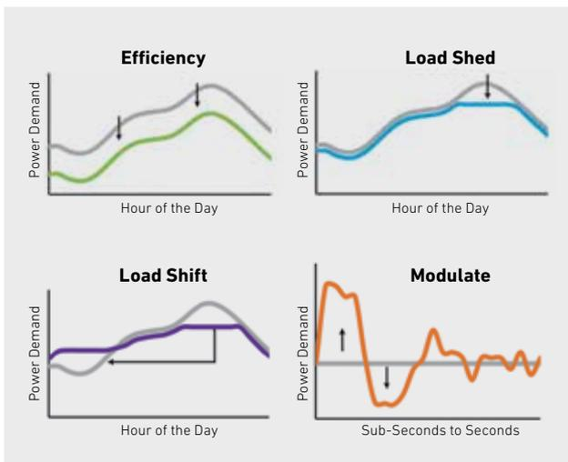
Building flexibility load curves – examples of load curve manipulation.
