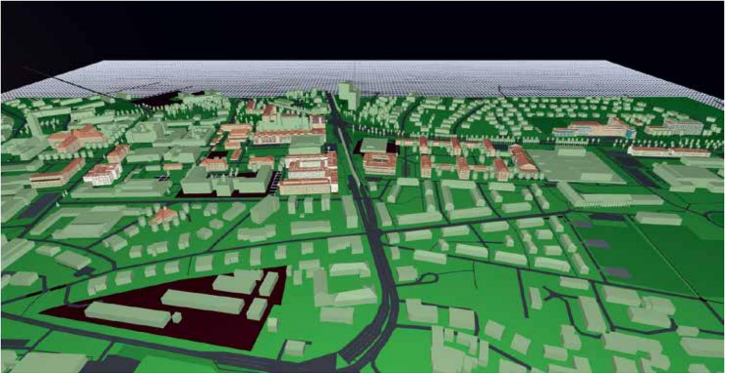
Illustration from a tool in the CHAMPS modelling platform, which highlights building complexes at a community scale that can be simulated for their combined heat, air, moisture and pollutant conditions, including an energy performance assessment.
