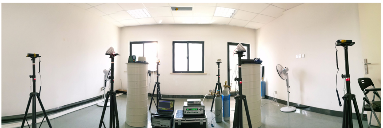
Indoor air quality monitoring in the P+ Experimental Building in Wujin, Jiangsu, P.R. China, comprising measurement of VOCs, PM 2.5 , thermal and humidity conditions, as well as energy performance.
