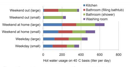
Figure 1. Domestic hot water usage pattern 'Corrected M-1 Mode' for 4-member family.
