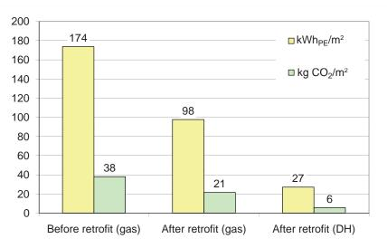
Figure 2. Karlsruhe-Rintheim neighbourhood refurbishment project - primary energy and  $CO_2$  emissions for heating and domestic hot water supply - before retrofit (measured)
