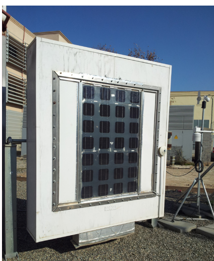
Figure 2. Measuring the thermal response of ventilated photovoltaic double skin facades under real climatic conditions.
