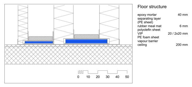
Figure 31: Vertical section of a cold (left) an a deep-freeze room (right)
