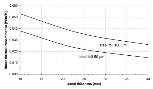
Figure 9: The effects of panel thickness and foil thickness on the linear thermal transmittance due to thermal bridging for a stainless steel foil ( $\lambda_{foi} = 25 \text{ W/(m·K)}$ ;  $\lambda_{cop} = 4 \cdot 10^{-3} \text{ W/(m·K)}$ ), based on numerical calculation
