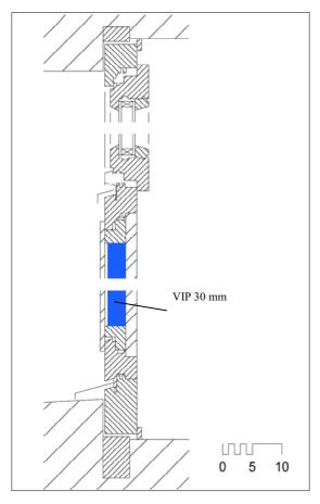
Figure 37: Parapet with VIP
