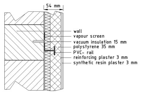
Figure 40: Cross-section of the insulated wall
