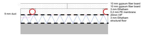
Figure 87: Principle construction layout of dry VIP based floor heating system (concept 2)
