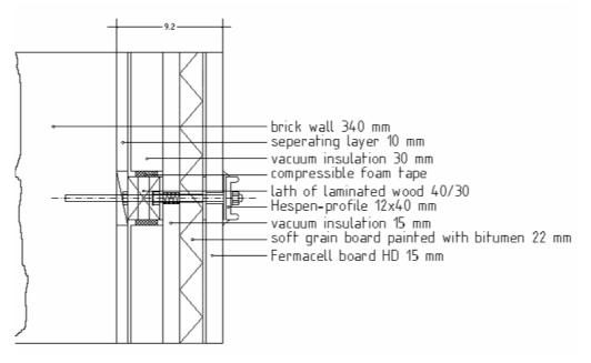
Figure 48: Cross-section of the northern wall
