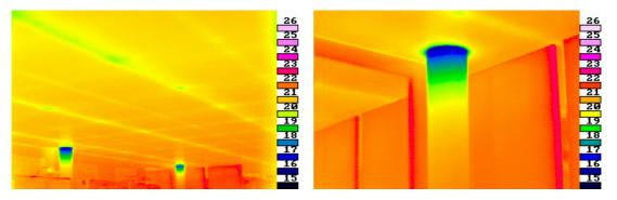
Figure 21: Concrete pillars passing from the roomside through the VIP-layer to the outside concrete roof slab. Pictures with the IR-Camera
