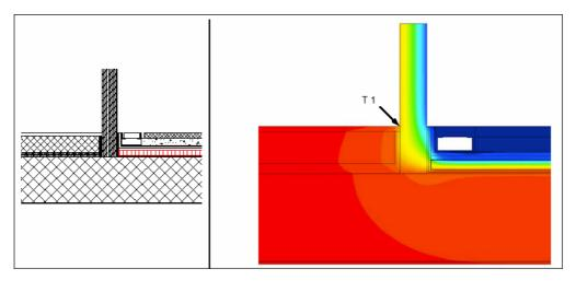
Figure 74: Vertical section through the terrace construction and threedimensional computational heatflow analysis. The calculated temperature T1 is 14 °C.
