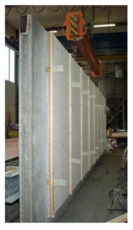
Figure 61: Left: Intended design for the prefabricated wall elements. An average U-value of 0.15  $W/(m^2 \cdot K)$  is achieved with a total thickness of only 27 cm. Right: Photo of a prefabricated wall element
