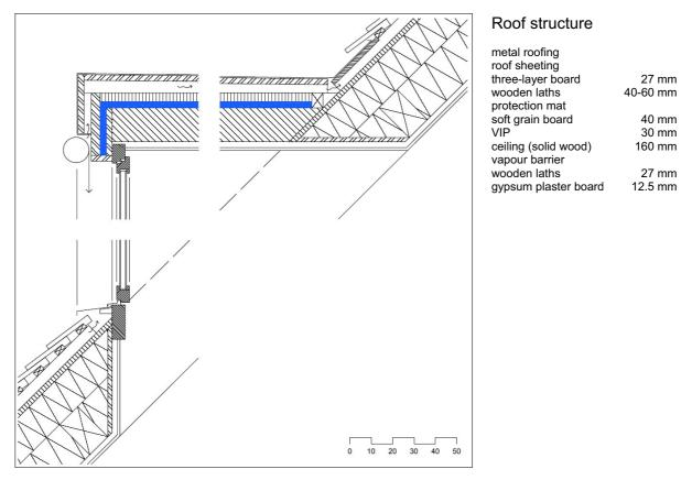
Figure 80: Vertical section through a prefabricated dormer window for the renovation of an old building
