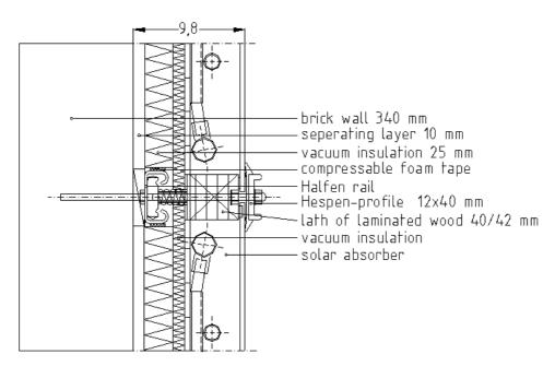
Figure 49: Cross-section of the south wall
