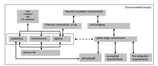
Figure 75: Relationships between different requirements for building panels with incorporated vacuum insulation panel.
