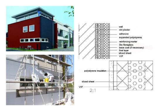
Figure 63: Left: View of the passive house with lined VIP. The black façade has conventional, 30 cm thick insulation to demonstrate the difference in thickness compared to the red façade insulated with VIP. Lined VIP being mounted onto the façade Right: Cross-section of the wall
