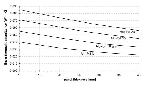
Figure 8: The effects of panel thickness and foil thickness on the linear thermal transmittance due to thermal bridging for an aluminium foil ( $\lambda_{foil} = 200 W/(m \cdot K)$ ;  $\lambda_{cop} = 4 \cdot 10^{-3} W/(m \cdot K)$ ), based on numerical calculation
