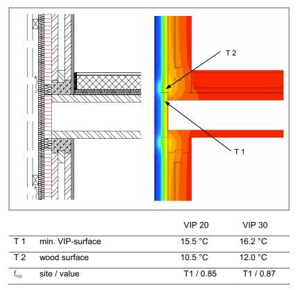
Figure 79: Vertical section through a joint of elements, three-dimensional computational heatflow analysis and calculated temperatures
