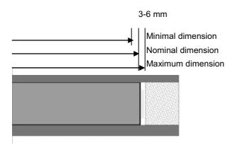
Figure 76: Tolerances in VIP integrated building components
