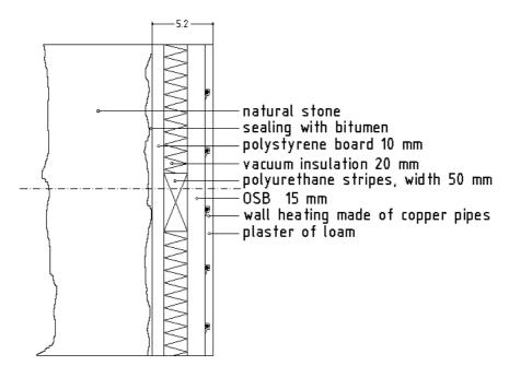
Figure 51: Cross-section of the wall
