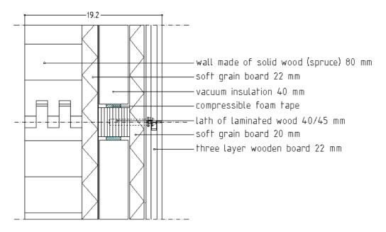
Figure 44: Cross-section of the northern wall
