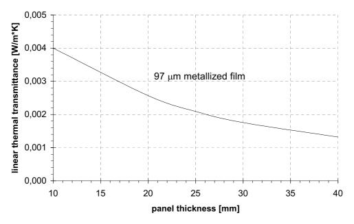
Figure 10: The effects of panel thickness on the linear thermal transmittance due to thermal bridging for a three layer metallized film;  $\lambda_{cop} = 4 \cdot 10^{-3} W/(m \cdot K)$ ), based on numerical calculation
