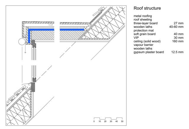
Figure 26: Section through the dormer window construction
