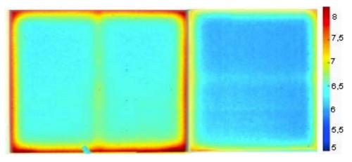
Figure 55: Infra-red image of two elements. On the left hand side the spacer is made of stainless steel and on the right hand side the spacer is made of Purenit.
