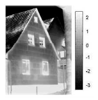
Figure 42: Infra-red image (from 2003) of the gable façade three years after the external thermal insulation composite system was installed. The edges of the VIP can be seen as lines (thermal bridges).
