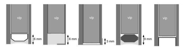
Figure 16: Different edge spacers. a.) aluminium spacer double-glazing; b.) sealant spacer; c.) reinforced non-metallic tape (0.15 mm); d.) optimised thermoplastic spacer (Henkel Tereson Thermoplastic Spacer); e.) polymer U-section
