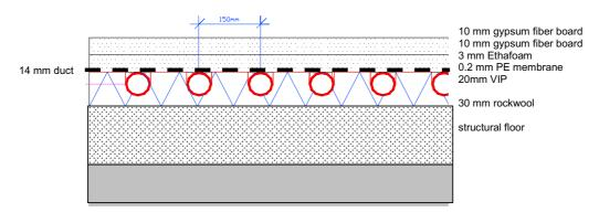
Figure 88: Principle construction layout of an acoustically improved dry VIP based floor heating system (concept 1)
