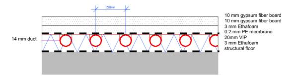
Figure 86: Principle construction layout of dry VIP based floor heating system (concept 1)
