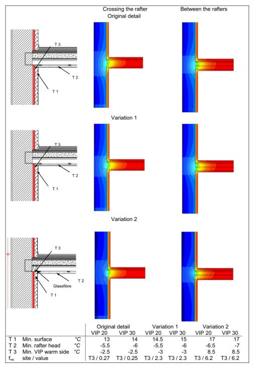
Figure 72: Three-dimensional computational heatflow analysis of the support of the ceiling
