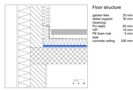
Figure 28: Vertical section through the joint detail at parapet
