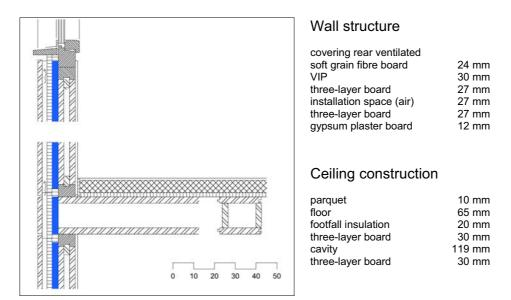
Figure 77: Vertical section through the window and the support of the ceiling
