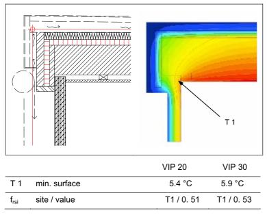
Figure 82: Vertical section through the dormer window, threedimensional computational heatflow analysis and calculated temperatures.
