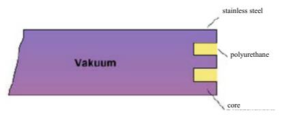
Figure 14: Section through a VIP. Sketch of the serpentine construction
