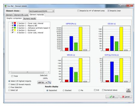
Figure 11 LCA comparison of a construction element's materials
