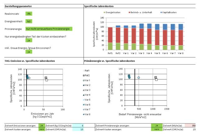
Figure 9 Screenshot from the Output sheet of the INSPIRE tool. As the main result, impacts of different renovation packages are shown with the graphs at the bottom. On the left-hand side, emissions are shown in relation to the life cycle costs for each renovation package; on the right-hand side, primary energy use is shown for each renovation package in relation to the life cycle costs.
