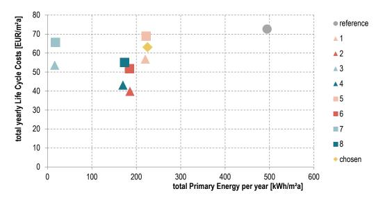
Figure 17 Results for the total primary energy for all the analysed renovation packages
