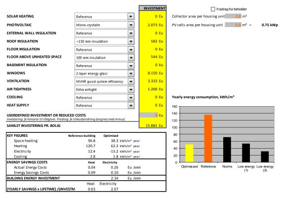
Figure 5 Example of ASCOT results for optimization of a building renovation with Annex56 methodology (Mørck, 2015)
