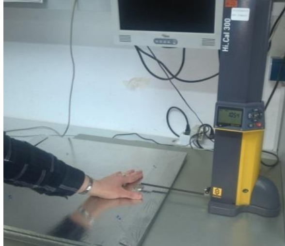
Figure 119: Setup for thickness determination on VIP with ME 1. Source: FIW München.
