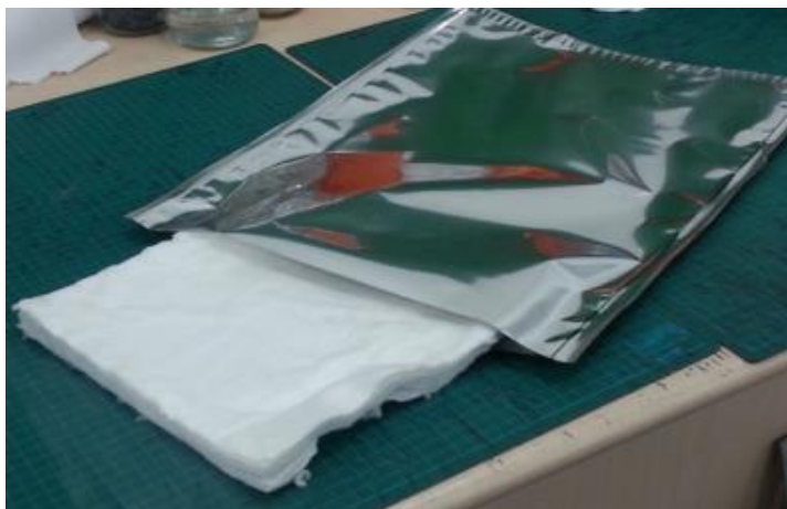
Figure 68: VIP before evacuation.
