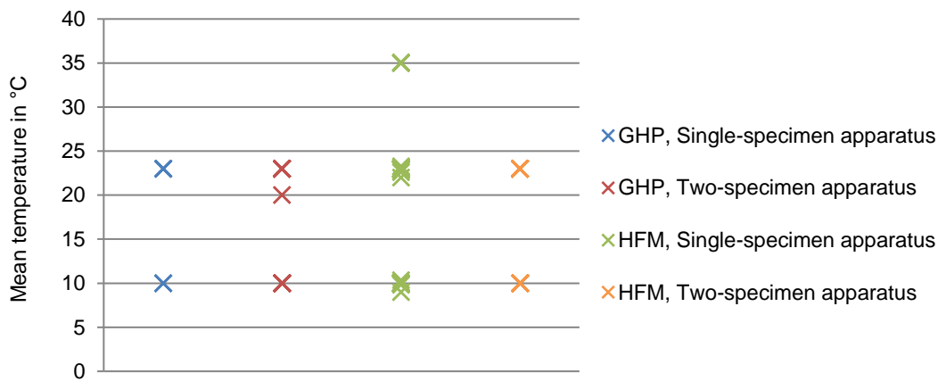
Figure 31: Applied mean temperature for thermal conductivity assessment distinct to type of apparatus.
