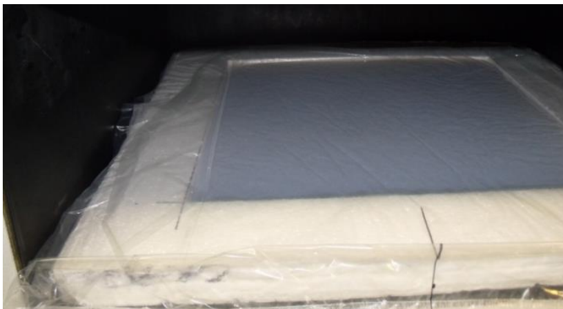
Figure 10: Self-made specimen holder for loose filled granulate made of EPS frame; the sample is sealed in a PE bag at ambient pressure. Source: Électricité de France.
