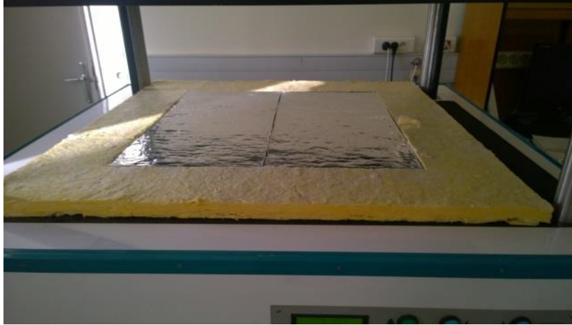
Figure 16: VIP in the heat flow meter apparatus with a guard of mineral wool around the specimen. Source: Centre Scientifique et Technique du Bâtiment.
