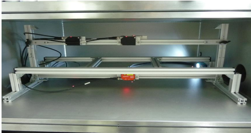
Figure 26: Equipment for determination of internal pressure measurement using the foil lift-off method in a vacuum chamber, laser measurement gauges are placed inside the vacuum chamber, VIPs are placed on a rectangular support with 250mm side length. Source: FIW München.
