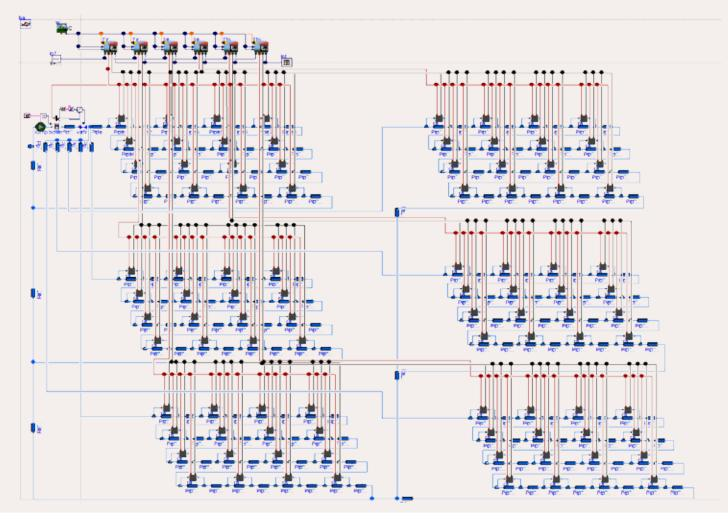
An object-oriented Modelica simulation model using the EBC Annex 60 framework technology. Source: RWTH Aachen University
