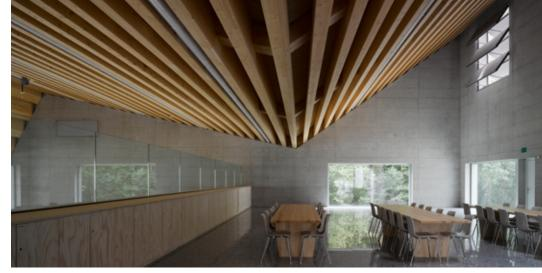
The gym and canteen at Saviese primary school in St-Germain, Switzerland, equipped with demand controled natural ventilation and a ventilative cooling system. The monitoring results show that four groups of openings, placed at the right positions and controlled with a simple BMS system, offer excellent indoor air quality and summer comfort without the presence of a single fan or duct. Source: Dominique Uldry
