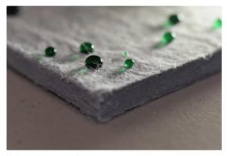
Hydrophobic aerogel fibre mat. Source: ASPEN AEROGEL
