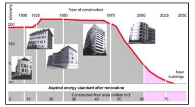
Energy consumption of Swiss residential buildings (Canton of Zurich) for different construction periods and the aspired-to energy standard for buildings constructed 1925 – 1990
