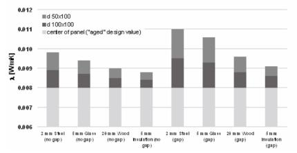
Figure 6:Thermal bridge edge effect of different adjacent materials on overall conductivity ( $\lambda_{eff}$ ) of a panel with MF-envelope and a center-of-panel conductivity of 8•10<sup>-3</sup> W/(m•K). "d 100x100" is the increase for a panel of 100x100 cm<sup>2</sup> compared to  $\lambda_{cop}$  and "d 50x100" is the increase for a panel of 50x100 cm<sup>2</sup> compared to the larger format.
