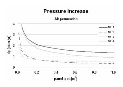
*Figure 2: Edge effect on internal pressure increase by air permeation through four different metallized films.*
