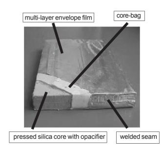
Figure 1: Components of a VIP. The core-bag provides mechanical stability for handling and protects the welding area from being polluted by core-powder (photo: va-Q-tec).
