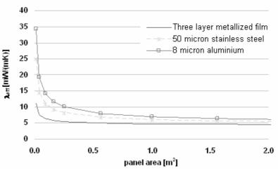
Figure 5: Thermal bridge effect of different envelope materials on overall conductivity ( $\lambda_{eff}$ ) of a panel with center-of-panel conductivity ( $\lambda_{\chi op}$ ) of 4•10<sup>-3</sup> W/(m•K).
