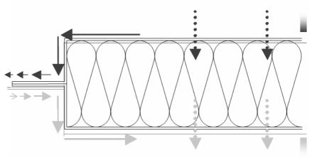
Figure 4: Schematic representation of a cold bridge caused by the VIP envelope.
