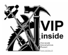
Figure 8: Draft sketch for an adhesive warning label to mark VIP panels and building components containing VIP.
