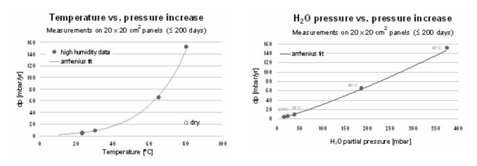
Figure 3: Internal pressure increase caused by water vapour permeation is proportional to the differences in the partial pressures inside and outside the panel. The measurements were done at room temperature after cooling down the samples for some hours.
